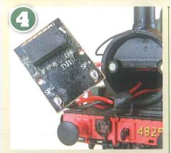
With the blanking plug removed, the 6-pin DCC socket and the speaker wire terminals can be dearly seen. Zimo's MX649 decoder was tried next, but wouldn't fit in the space available below the smokebox weight so we changed tack.
