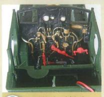
Removal of the cab reveals the interior plus the lower rear cab bulkhead and the oulding to locate the speaker.
