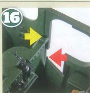
The cab features doors which can be positioned open or dosed. In order to facilitate reassembly, note the way in which the door pivots (upper one arrowed in red), and are engaged with holes in the cab floor and the ends of the lower cab bulkhead (arrowed in yellow).
