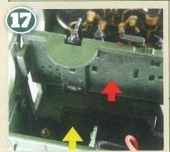
The lower cab rear bulkhead (arrowed in red) is normally held in position by the cab moulding so no additional fixing is required. It can therefore be lifted dear, in turn releasing the speaker locating moulding (arrowed in yellow).
